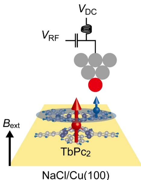
Fig.1 Schematics of the experimental setup. A single  $\text{TbPc}_2$  molecule adsorbed on a 2 ML  $\text{NaCl}/\text{Cu}(100)$  surface is studied using ESR-STM with an out-of-plane external magnetic field.
