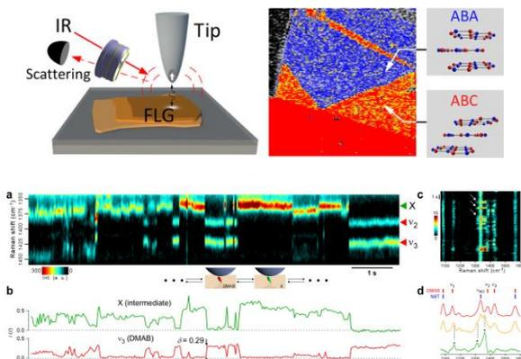
(top) the infrared nanoscopy imaging of trilayer graphene; (bottom) time-dependent SERS spectra of single-molecule dimercapto-azobenzene reaction intermediates
